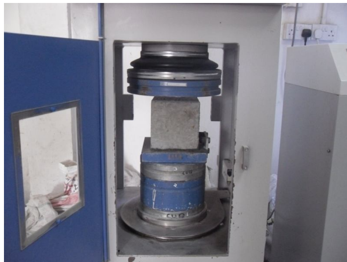
Plate 2.1: Cube inside Compressive Strength Machine
